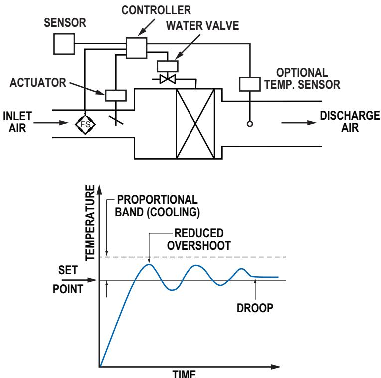
**Figure 5.4** Constant-Volume Reheat Air Terminal Unit with Proportional Control
