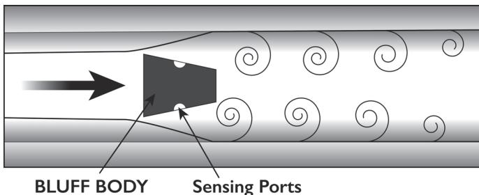
**Figure 6.2** Bluff Body in Airflow
