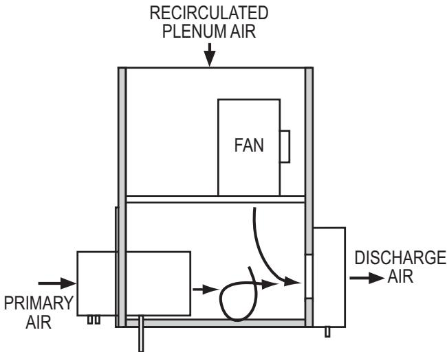
**Figure 3.4** Parallel Air Terminal Unit Configuration
