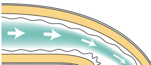
**Figure 6.10 Overstretched Bend at Inlet**
