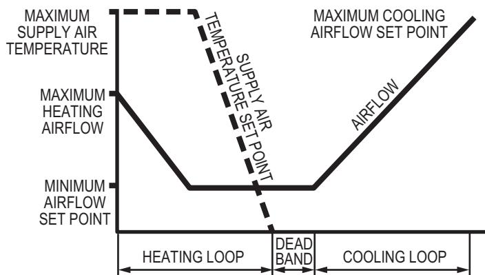
**Figure 5.9** Throttling Variable-Air-Volume Terminal Unit—
