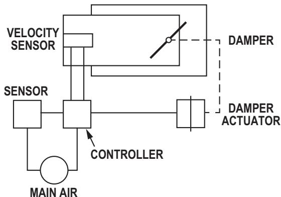
**Figure 5.2** Pressure-Independent Air Terminal Unit
