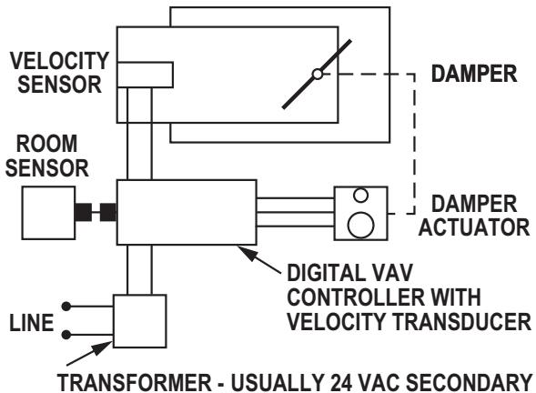
**Figure 2.13** Direct Digital Control Pressure-Independent Control Diagram
