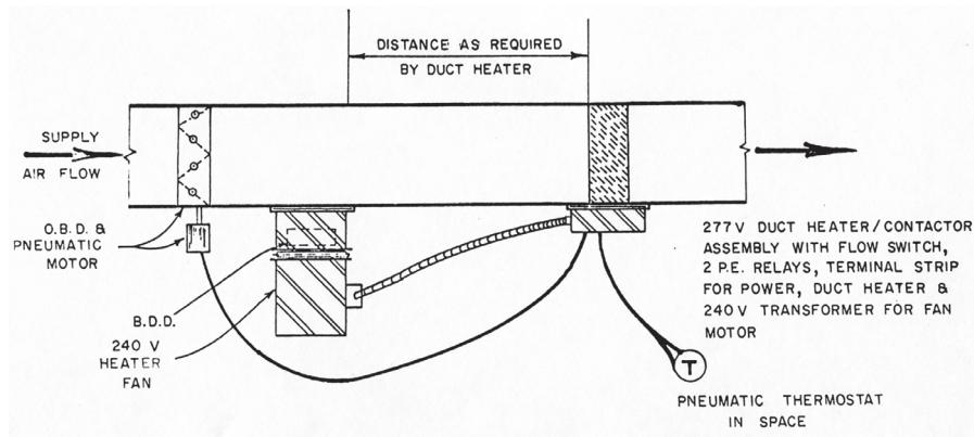
**Figure 3.1** Exterior Zone Variable-Air-Volume Arrangement
