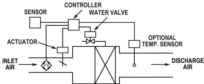
**Figure 5.3** Constant-Volume Reheat Air Terminal Unit
