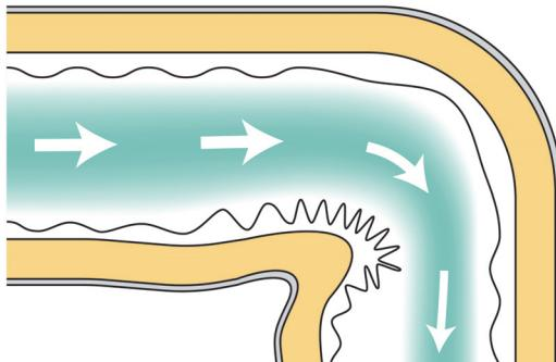
**Figure 6.8 Poor Flex Elbow**
