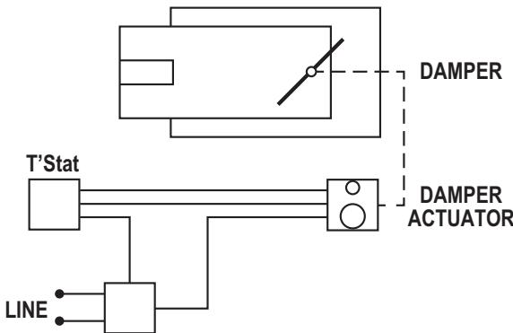
**Figure 5.1** Pressure-Dependent Air Terminal Unit
