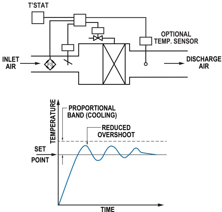
**Figure 5.5** Constant-Volume Reheat Air Terminal Unit
