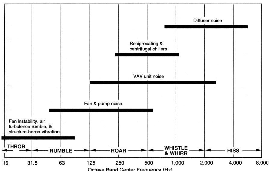
**Figure 4.2** Frequency Ranges of Typical Indoor Noise Sources
