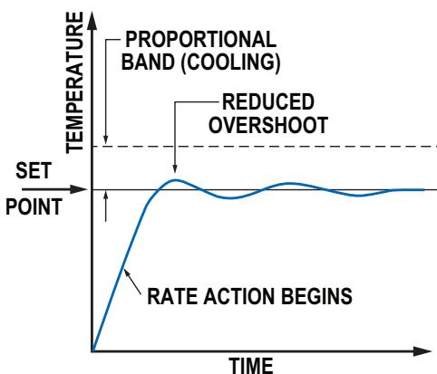
**Figure 5.6** Constant-Volume Reheat Air Terminal Unit with Proportional plus Integral plus Derivative Control
