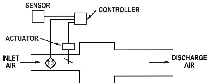
**Figure 5.8** Throttling Variable-Air-Volume Terminal Unit
