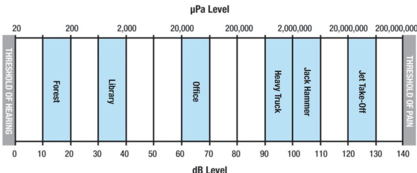
**Figure 4.4** Representative Sound Pressure Levels
