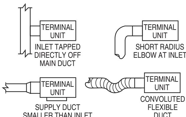
Figure 6.6 Typical Poor Inlet Conditions
