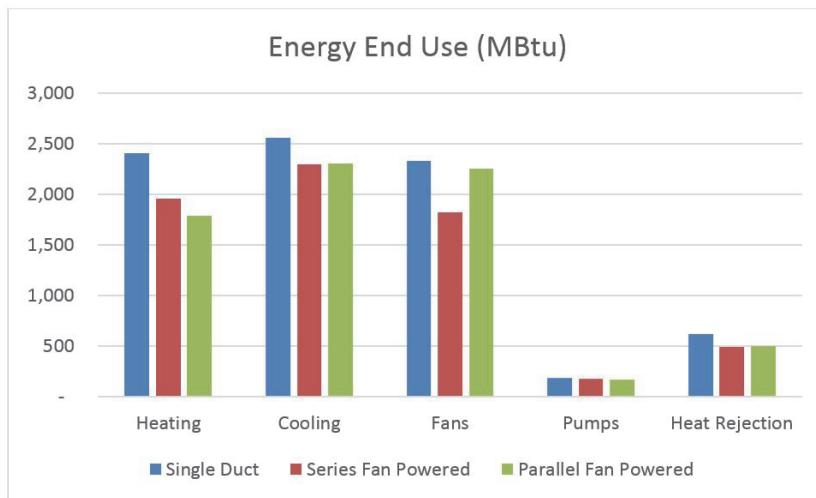
Figure 8.5 Annual Mechanical System Energy Use in Climate Zone 3A (Atlanta)
