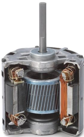
**Figure 6.4 Permanent Split Capacitor Motor**
