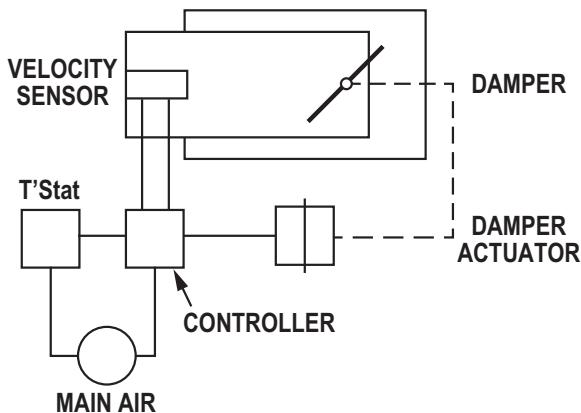
**Figure 2.11** Pneumatic Pressure-Independent Control Diagram
