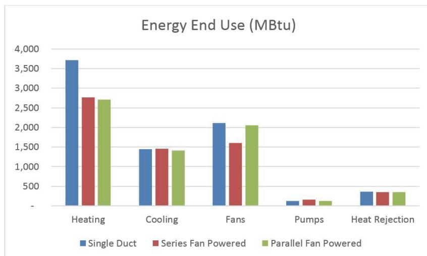
Figure 8.6 Annual Mechanical System Energy Use in Climate Zone 5A (Chicago)
