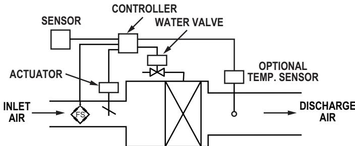
**Figure 5.7** Single-Duct, Constant-Volume Zone Reheat
