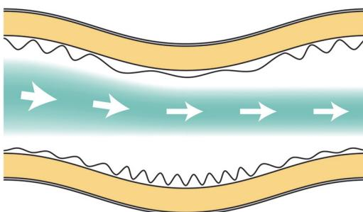
**Figure 6.9 Sagging Flex Duct**
