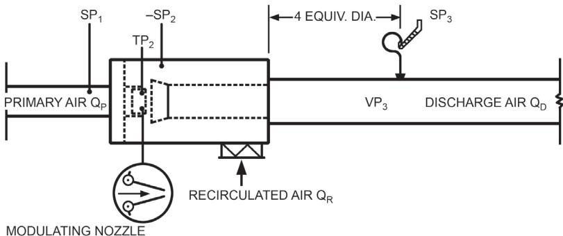
**Figure 2.5** Air-to-Air Induction Air Terminal Units
