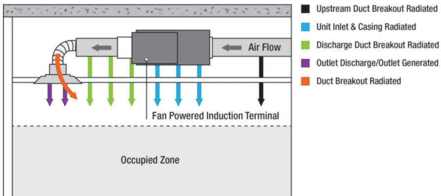
**Figure 4.12** Fan-Powered Terminal or Induction Terminal Acoustic Model
