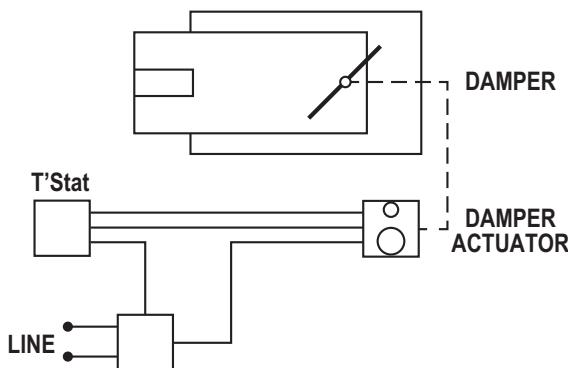
**Figure 2.10** Electric Control Pressure-Dependent Diagram
