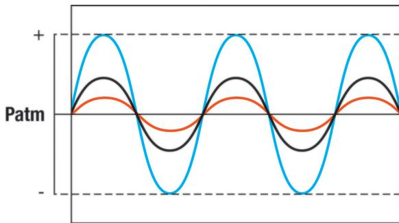
**Figure 4.3 Pure Tone with Varying Amplitude**
