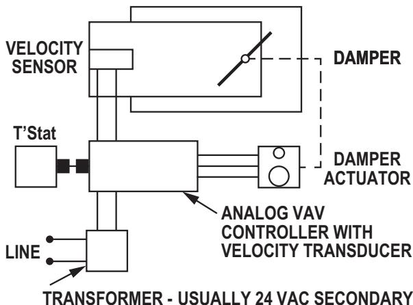
**Figure 2.12** Analog Electronic Pressure-Independent Control Diagram
