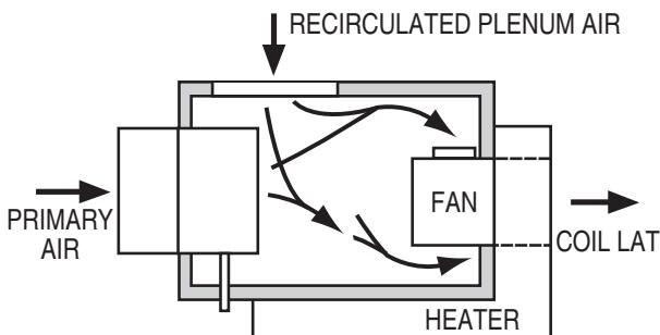
**Figure 3.5** Series Fan-Powered Air Terminal Unit Configuration
