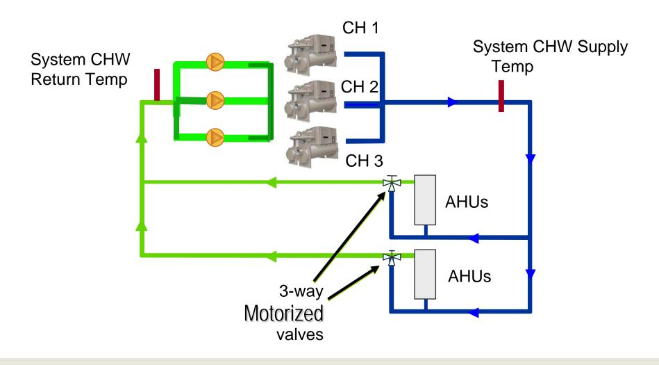
Don't switch off pumps even if chiller one/two chillers are off
