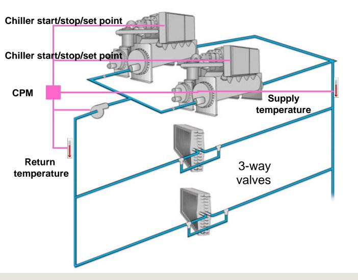
Change chiller set point to regulate the load and have a control on energy consumed
