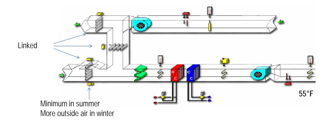
Economizer mode: Using outside air for cooling rather than mechanical cooling.
