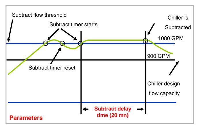
Based on Flow in the Bypass Line if # of chillers are more than SIX . . In a chiller plant
