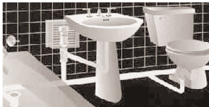
AIR ADMITTANCE VALVE BEHIND SINK
