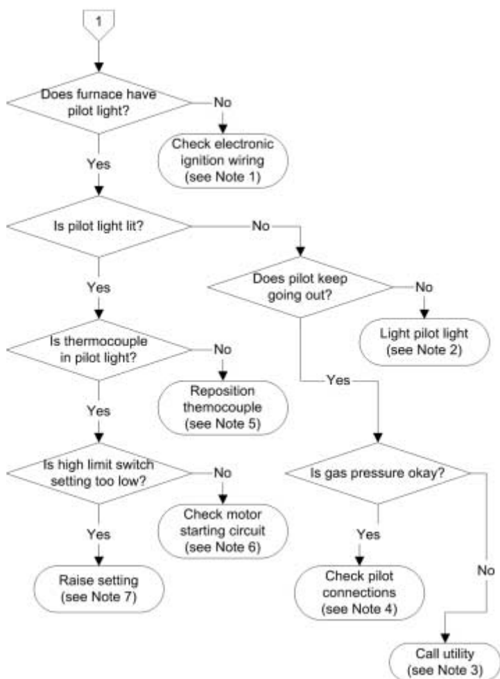
FIGURE 18.5 (continued) Troubleshooting flow chart for non-starting furnace.
