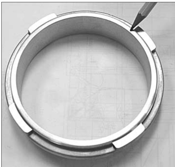
FIGURE 6.32 Check valve seat for wire draw, pitting, dirt, breaks, or erosion.
