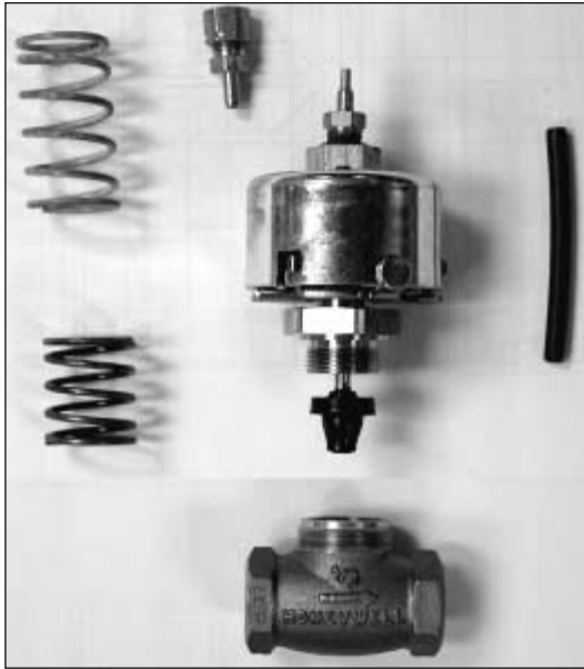
FIGURE 6.23 Valve rebuild kit showing different springs available.
