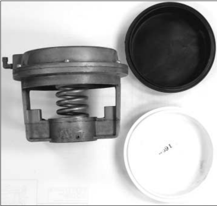
FIGURE 12.5 Pneumatic steam valve actuator with rubber (top) and silicone (bottom) diaphragms.
