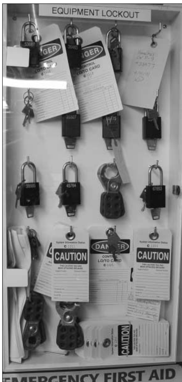
FIGURE A.1 Lock-out/tag-out center.
