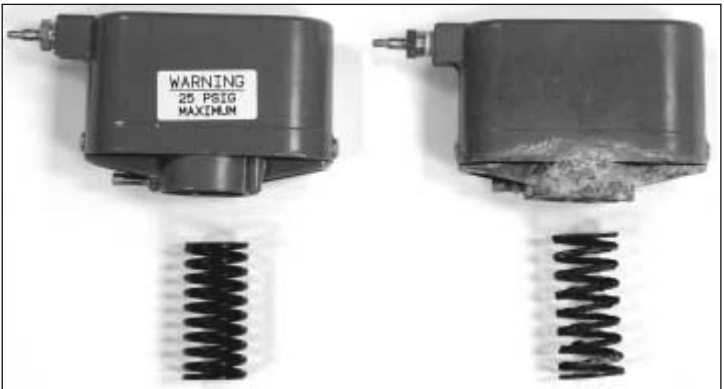
FIGURE 6.28 New (left) and corroded (right) valve actuator and spring.
