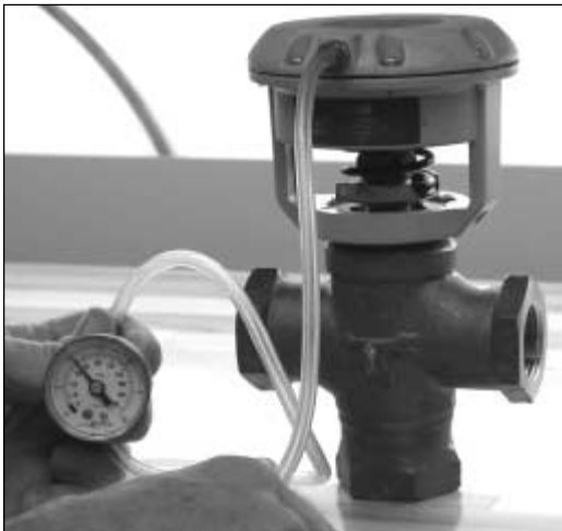
FIGURE 12.19 Squeeze bulb on pneumatic valve.
