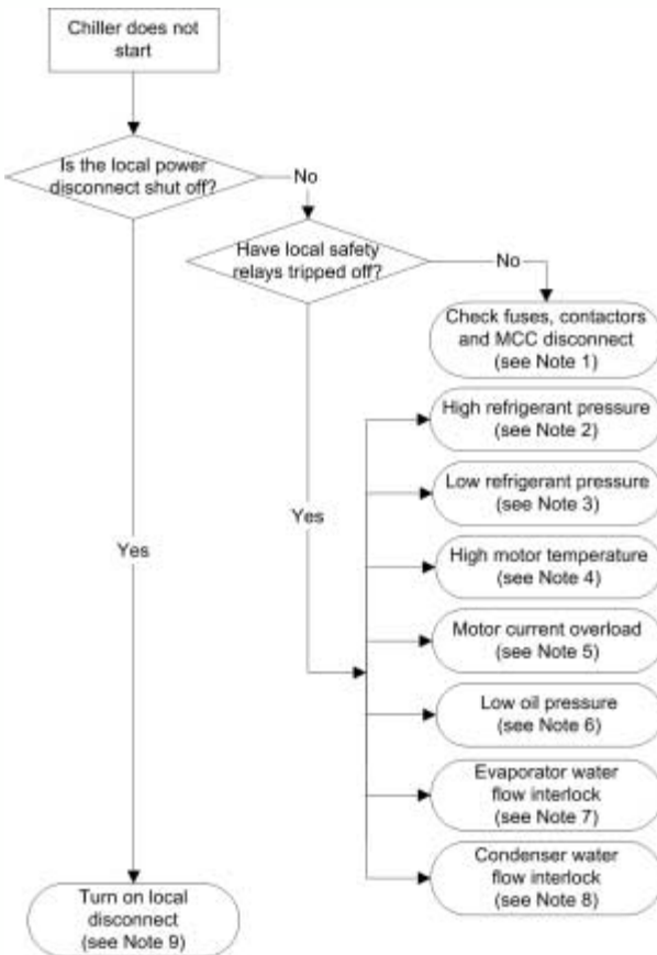
FIGURE 8.16 Chiller start-up troubleshooting flowchart.
