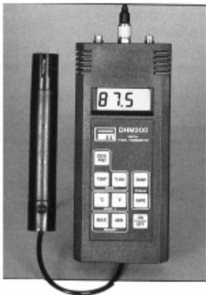
Figure 13-2. Electronic Temperature/Humidity/Dew Point Meter with Digital Readout. A hand-held electronic instrument with simultaneous digital readout of temperature and relative humidity or temperature and dew point. (Courtesy Mitchell Instrument Co.)
