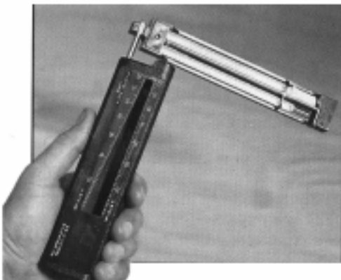
Figure 13-6. Sling Psychrometer with glass thermometer. (Courtesy Mitchell Instrument Co.)
