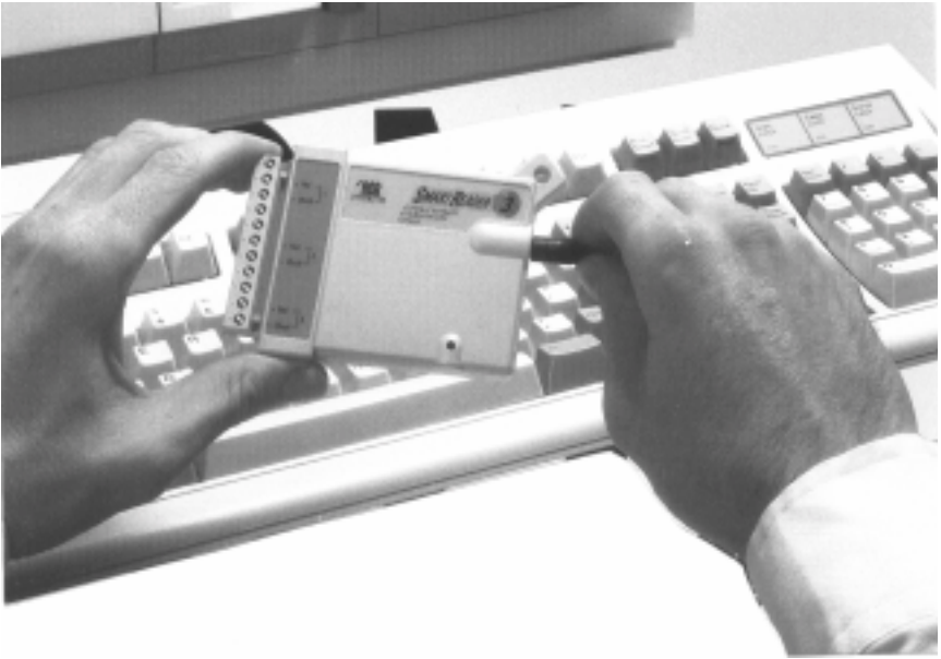
Figure 13-3. Electronic Data Loggers have on-board temperature and humidity sensors or with remote sensors for temperature, pressure, electric current flow, or pulse signals. (Courtesy ACR Systems Inc.)
