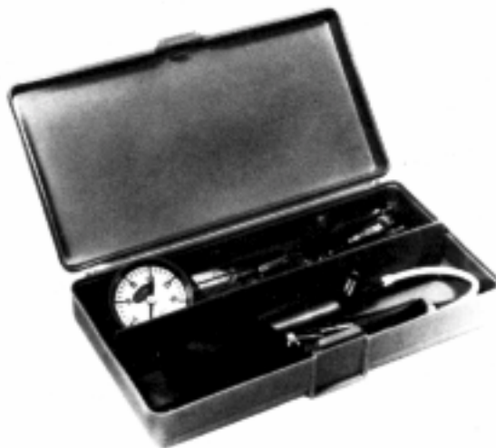
Figure 13-20. Pneumatic Control Calibration Kit. A typical calibration kit. (Courtesy Barber-Colman.)
