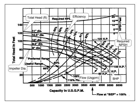
Figure 11 shows a typical pump curve. Since pumps are direct drive, the pump curves are typically for standard motor speeds (1200, 1800 or 3600 rpm). The required flowrate and head can be plotted and the subsequent efficiency and impeller diameter can be found. As the flow increases, generally the Net Positive Suction Head (NPSH) decreases. This is due to the increased fluid velocity at the
