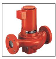
Typically centrifugal type pumps are used for both condenser water and chilled water systems. They can be either inline or base mounted. The pumps must be sized to maintain the system dynamic head and the required flow rate. Normally, the pumps are located so they discharge into the chiller heat exchangers.
