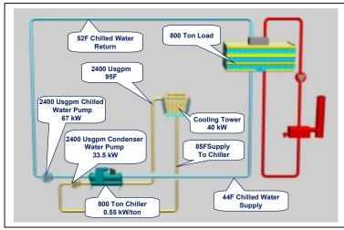
Figure 35 – Basic Single Chiller System Operation
