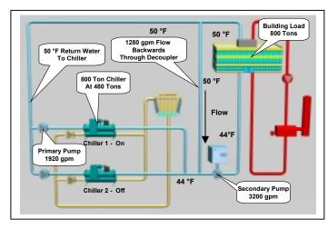
Figure 70 - Primary/Secondary Loop at Low Delta -T
