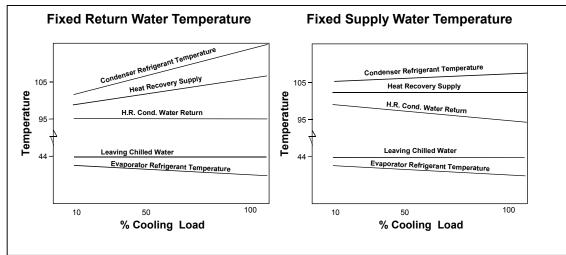
Figure 63 - Heat Recovery Chiller Control Options
