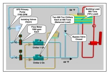
Figure 66, - Basic Variable Primary Flow Operation
