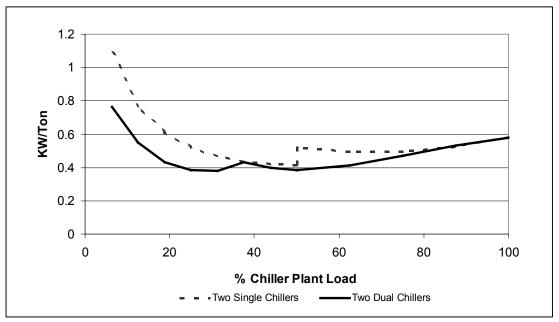
Figure 32 - Chiller Performance Vs. Plant Load
