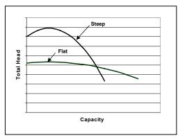
Figure 10 shows a steep and flat curve profile. Different pumps provide different profiles each with their own advantages. The steep curve is better suited for open systems such as cooling towers where high lift and stable flow are desirable. The flat profile is better suited for systems with control valves. The flat profile will maintain the necessary head over a wide flow range.
