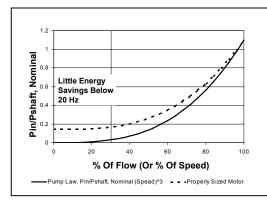
Figure 13 shows percent pumping power as a function of percent flow. From this figure, it can be seen that VFD pumps will not save much energy below 33% or 20Hz. Operating pumps much below 30% starts to create problems for motors, chiller minimum flows, etc. Since there are minimal savings anyway, the recommended minimum frequency is 20 Hz.
