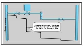
Figure 22 shows typical pressure drops from the supply to the return line for a cooling coil. For a modulating valve, the valve pressure drop should be as large a percentage as possible when compared to the system pressure drop; preferably over 50%. The reason is to maintain valve authority. For on-off control, any valve can be used as long as it can pass the required flow rate with the pressure differential available.
