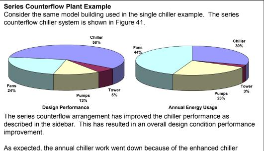
As expected, the annual chiller work went down because of the enhanced chiller performance. On the other hand, the large condenser pump (sized for the design condenser flow) which must operate whenever there is a need for chilled water, has increased the annual pump work. Whether series counterflow will save energy on an annual basis will depend on the pump penalty vs. the chiller savings.
