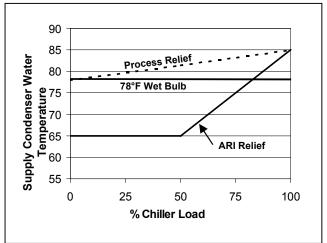
Figure 74 - ARI 550/590 vs. Process Condenser Relief
