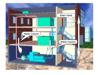
The piping is usually steel, copper or plastic. The chilled water piping is usually a closed loop. A closed loop is not open to the atmosphere. Figure 3 shows a simple closed loop with the pump at the bottom of the loop. Notice that the static pressure created by the change in elevation is equal on both sides of the pump. In a closed loop, the pump needs only to overcome the friction loss in the piping and components. The pump does not need to "lift" the water to the top of the loop.
