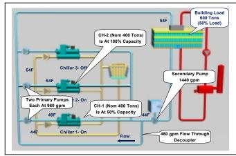
Relocating the decoupler can make sense if one or more of the chillers is a dual compressor model. The dual compressor chiller has very good part load performance. Single compressor chillers typically work best when fully loaded. By locating the dual compressor chiller close to the decoupler line and the single compressor chiller furthest away, the strengths of each chiller can be maximized. Another application for backloading chillers is where one of the chillers is a heat recovery
