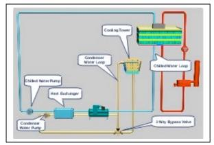
Figure 55 shows a different free cooling arrangement with the chiller in series with the heat exchanger. Since the heat exchanger operates with a higher return chilled water temperature, the operating season is longer than the parallel arrangement, offering more annual savings. This is an integrated system with the chiller "trimming" the chilled water temperature while operating with significant condenser water relief. Because the heat exchanger is piped directly in series with the chiller, the
