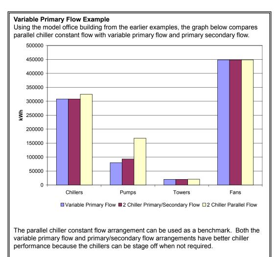
The major savings comes from reduced pump work. The pumps are smaller (flow is based on design load rather than connected load) and the flow varies with the load.
