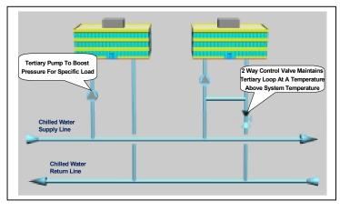
There are two key applications where tertiary piping is helpful. The first is where the pressure available in the secondary loop is not sufficient for a specific load. The second is where a load requires a different temperature range than the main system.
