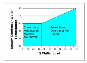
Minimum chiller setpoints are not a specific temperature. They change depending on the chiller load. A conservative number such as 65°F is recommended.
