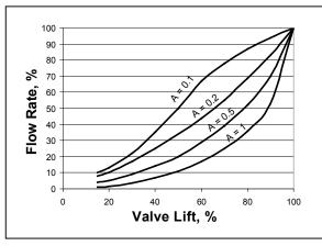
Figure 23 shows the change in the valve characteristic that occurs at different Valve Authorities. Since the goal is to provide a valve with a performance characteristic that is the opposite of a coil characteristic (See Figure 21), it is important to maintain Valve Authority above 0.5.
