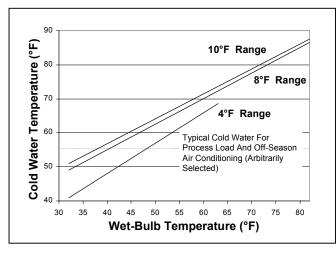
Figure 57 - Cooling Tower Performance Curve at Standard Conditions
