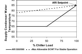
If aquastats are going to be used, then a lower setpoint than 85°F should be used. One recommendation is to set the aquastat at the minimum condenser water temperature acceptable to the chiller. The cooling tower will then operate at maximum fan power and always provide the coldest possible (based on load and ambient wet bulb) condenser water to the chiller until the minimum setpoint is reached. Then the tower fan work will stage down and maintain minimum setpoint.
