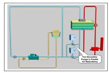
Secondary pumps are variable flow and sized to provide flow throughout the chilled water plant. In a sense, they handle all the pressure drops "outside the mechanical room". Refer to *Variable Flow Pumps*, page 13 on how to vary the flow through pumps.
