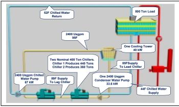
Figure 41 - Series Counterflow System Design
