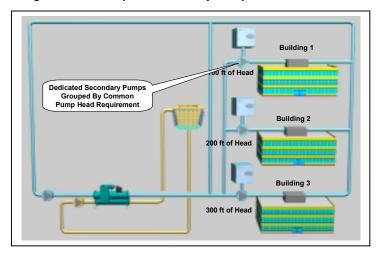
Figure 46 shows dedicated pumps for various loops. Multiple loops can serve areas with different operating schedules or widely different fluid pressure drops (such as a building on the far side of a campus). The individual loops can be scheduled off when not required. A good system design should always group loads with common pressure drop and scheduling requirements to reduce pumping work.
