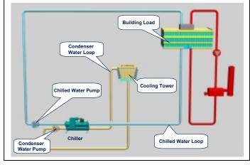
can be remote from the condensing section on air-cooled units. This has the advantage of allowing the chilled water loop to remain inside the building envelope when using an outdoor chiller. In applications where freezing conditions can be expected, keeping the chilled water loop inside the building avoids the need for some form of antifreeze.
