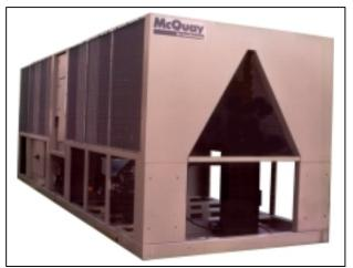
Many small to medium chiller plants use air cooled chillers with air-cooled screw chillers being common in the 150 to 400ton range. Air-cooled screw chillers offer very good performance particularly at part load. The compressors are modulating rather than stepped which provides more accurate control.
