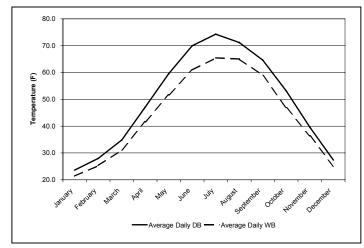
Figure 28 - Annual Ambient Drybulb Vs. Wetbulb
