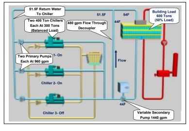
Figure 42 - Basic Primary/Secondary System Operation (50% Load)
