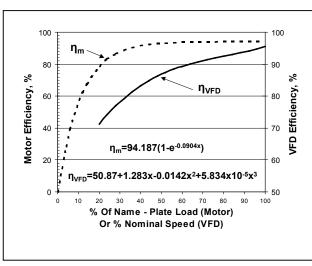
When both motors and VFDs operate at less than 100% capacity, their efficiency drops off. Figure 14 shows motor and VFD efficiencies at part load. It can be seen that oversizing motors can lead to significantly poorer performance than expected.
