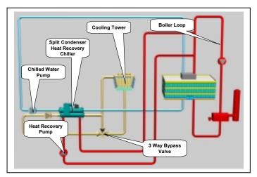
Figure 62 - Split Condenser Type Heat Recovery
