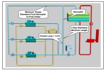
To avoid thermal contamination, the decoupler should be at least three pipe diameters in length. Longer decouplers tend to increase the pressure drop. When the secondary return flows straight through in the tee to the primary return, there should be at least 10 pipe diameters to the first chiller. This is to help avoid the possibility of having stratification in the primary return line, which can lead to unmixed water to the first chiller. This can lead to chiller cycling.
