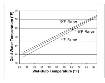
Figure 58 shows a cooling tower optimized for free cooling. The cooling tower was selected to provide  $48^{\circ}$ F condenser water at a  $45^{\circ}$ F wetbulb and  $4^{\circ}$ F range (50% building load). This allows 50°F chilled water to be produced.
