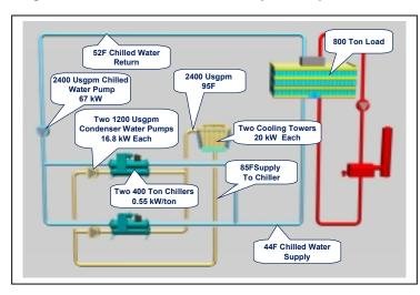
Figure 37 – Basic Parallel Chiller System Operation
