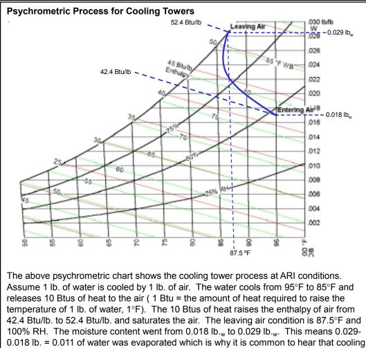
0.018 lb. = 0.011 of water was evaporated which is why it is common to hear that cooling towers lose about 1% of their water flow to evaporation. The latent heat of vaporization for water at 85°F is about 1045 Btu/lb. Multiplying the latent heat times the amount of evaporated water (1045 x 0.011) results in 11.45 Btus of cooling effect. Cooling the water required 10 Btus, the rest was used to cool the air sensibly. The air entered the tower at 95°F and left the tower at 87.5°F.
