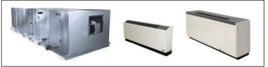
Chilled water coils are used to transfer the heat from the building air to the chilled water. The coils can be located in air handling units, fan coils, induction units, etc. The air is cooled and dehumidified as it passes through the coils. The chilled water temperature rises during the process.
